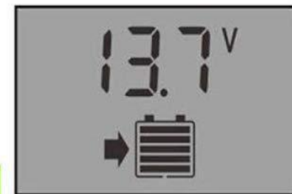
② Float Voltage
